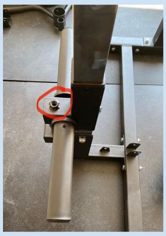
Slide weight holding attachment onto silver bar and keep the bolt side facing up
